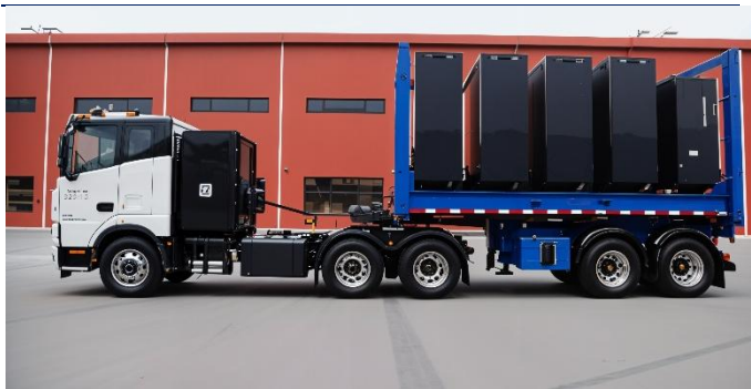
Figure 27: Pure One battery swap trailer
